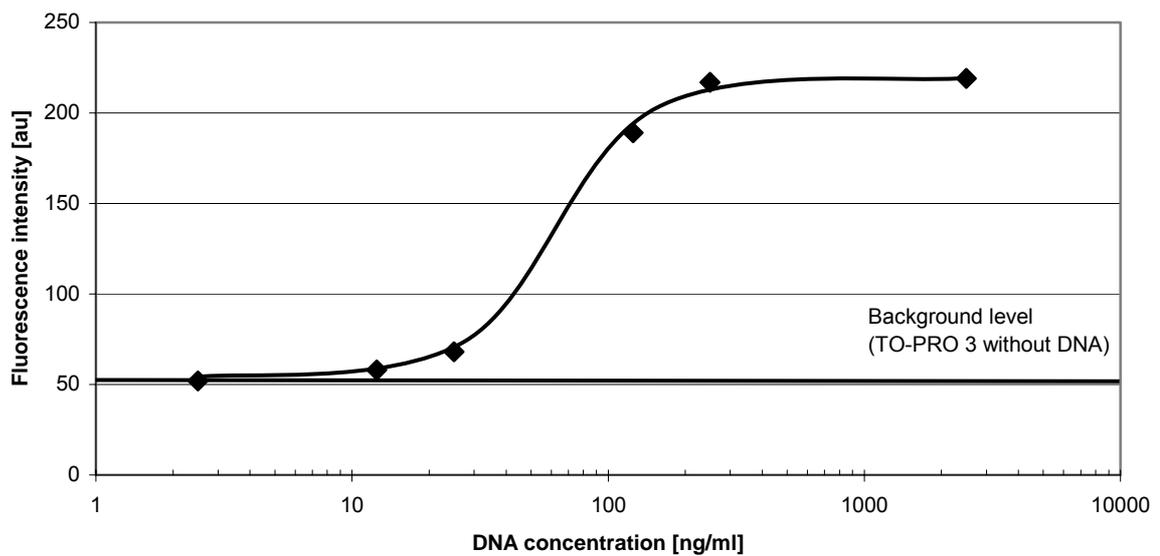
Figure 5. Fluorescence intensity as function of DNA concentration
