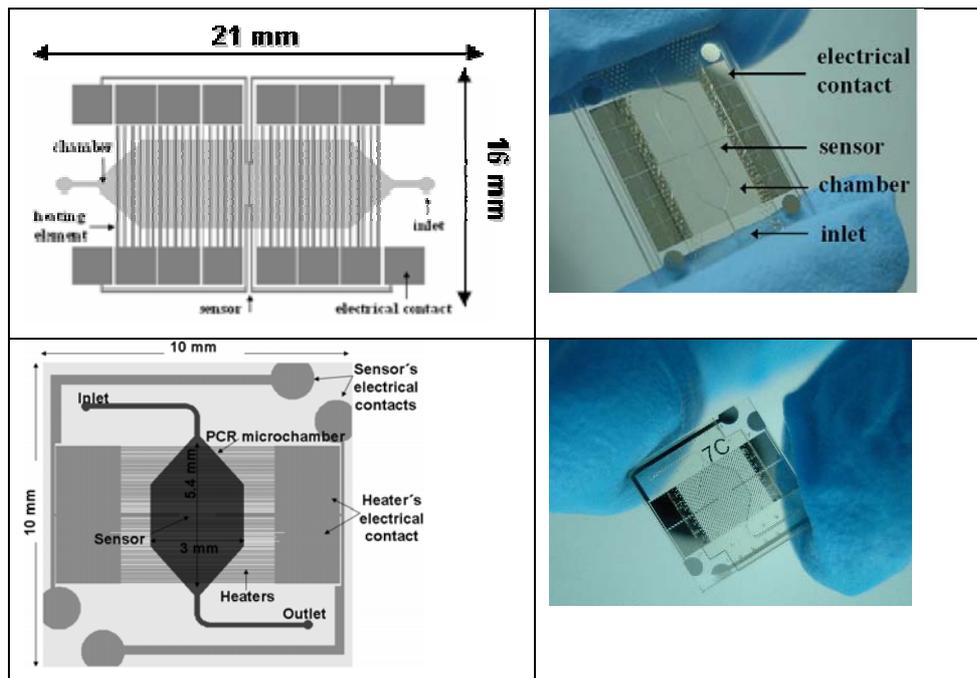
Figure 7. Comparison of the first year and second year chip Left) Schematic top view of the SU-8 chip. It consists of a rhombus shape microchamber, a resistive Ti/Pt sensor and two parallel heaters; Right) Picture of the chip
