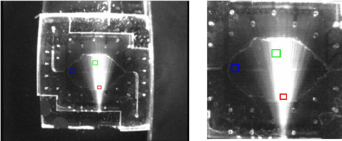
Figure 4. The chip at tests (left) and enlarged PCR chamber sector. Areas of analysis justified by the software marked with squares.
