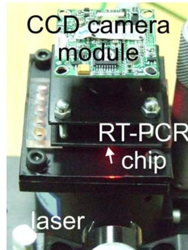
Figure 3. The measurement set-up with IKERLAN chip and side-wall edge coupling of laser light: a) scheme, b) view of the stand, c) detail of the stand – the CCD module positioned a few millimetres above the chip
