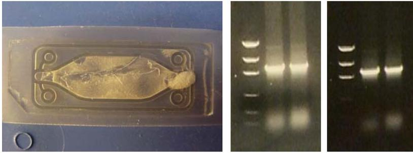
**B) Freeze-dried and PCR on “Close” chip from IKERLAN**
