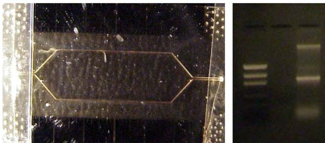
**Figure 2. On chip Freeze-dried PCR mixture: in A) “open” chip and in B “close” chip and PCR results**
