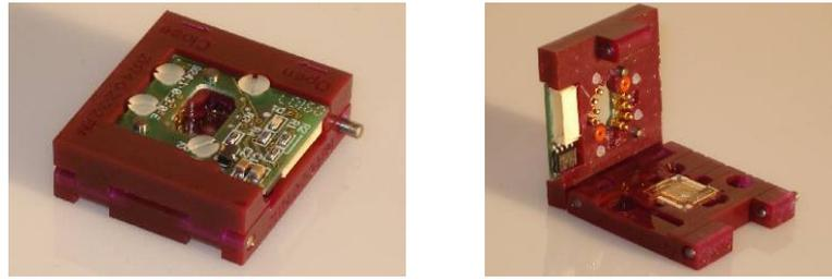
Figure 8. Photographs of the fabricated PCR microdevices: closed and open packaged device.
